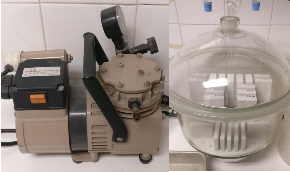
Figure 16 – Desiccator used in the porosity testing (on the right) and the attached compressor (on the left) utilized to control air pressure inside the vacuum recipient.
