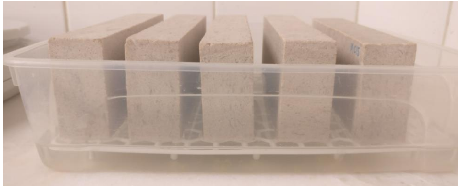
Figure 17 – Water absorption test, with the sample's surfaces on the supporting tray, 3 mm deep in water.
