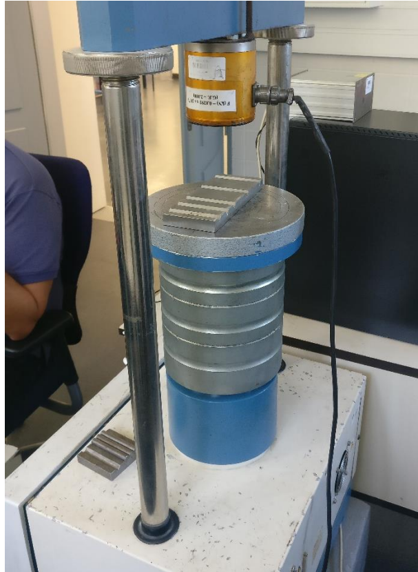
Figure 22 – DIGITAL TRITEST, from ELE, and the respective loading cell on top, utilized in the determination of sample failure load in natural stone samples with 10 mm and 20 mm thickness.
