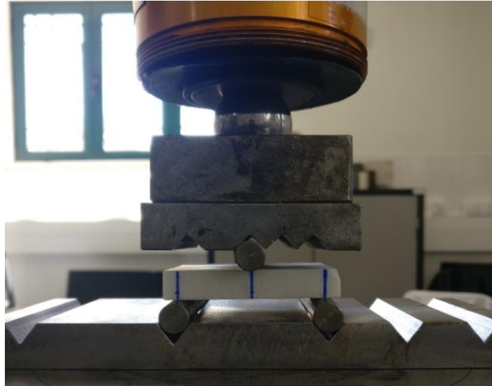
Figure 23–Setup for the flexural strength testing on the DIGITAL TRITEST soil press, for a 60x50x10 mm RC Marble sample, with two supporting rollers separated at a distance equivalent of 5 times the samples thickness, and a pressing roller in the middle.
