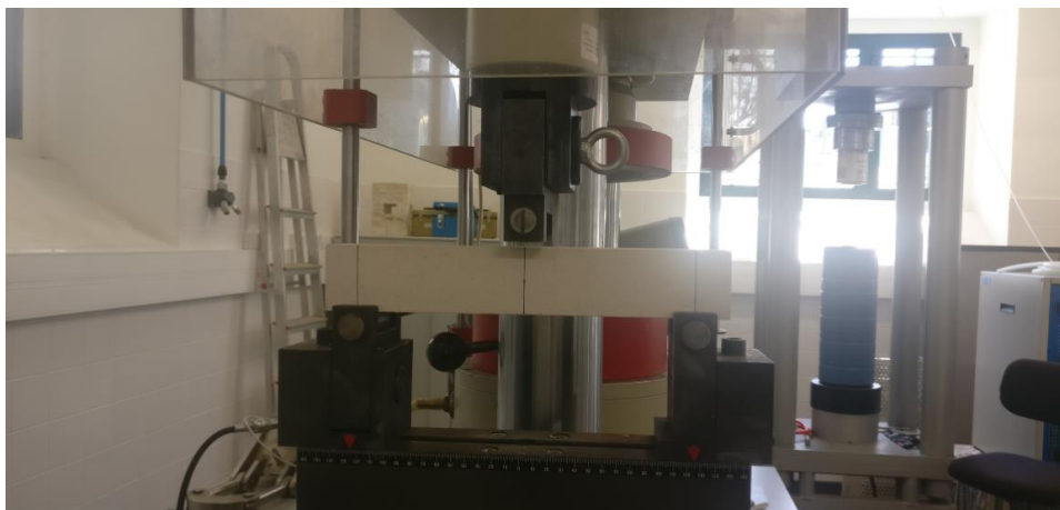
Figure 25 – Placement of a 300x50x50 sample on the FORM-TEST LEHRSYSTEME 506/1000/200 D hydraulic press, in which it was possible to set the desired distance, for the bottom rollers, thanks to its integrated ruler.
