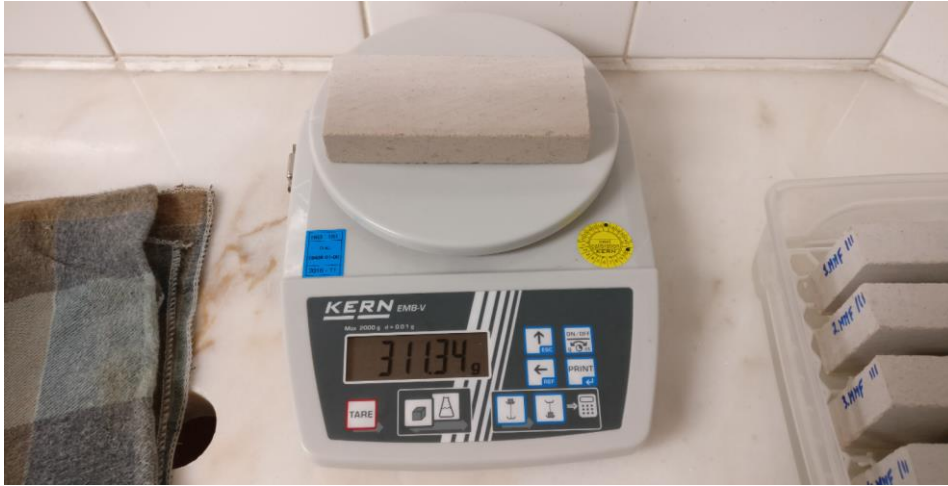
Figure 18 – Weighing process in the water absorption test, where samples were first cleared of excess water in the contacting surface, before being weighed and placed back into the container.
