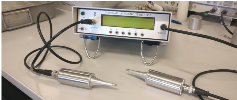
Figure 19 – Ultrasonic testing equipment (Steinkamp Ultrasonic Tester BP-7) with the correspondent pair of exponential transducers, with 45 Hz frequencies.
