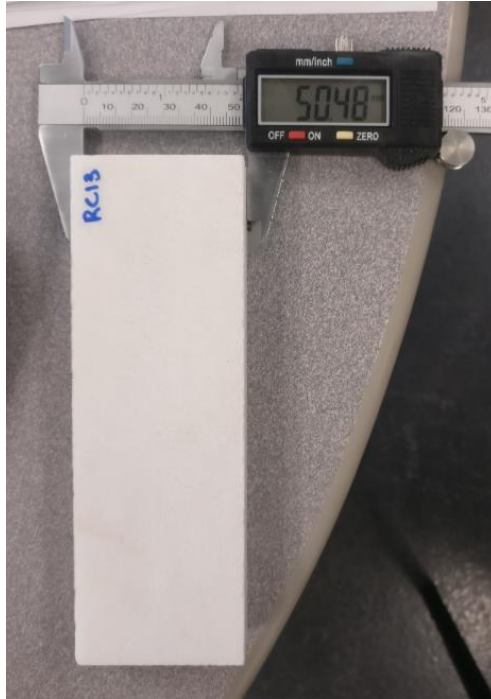
Figure 12 – Application of the digital caliper in the measuring of width on Marble RC13 sample.
