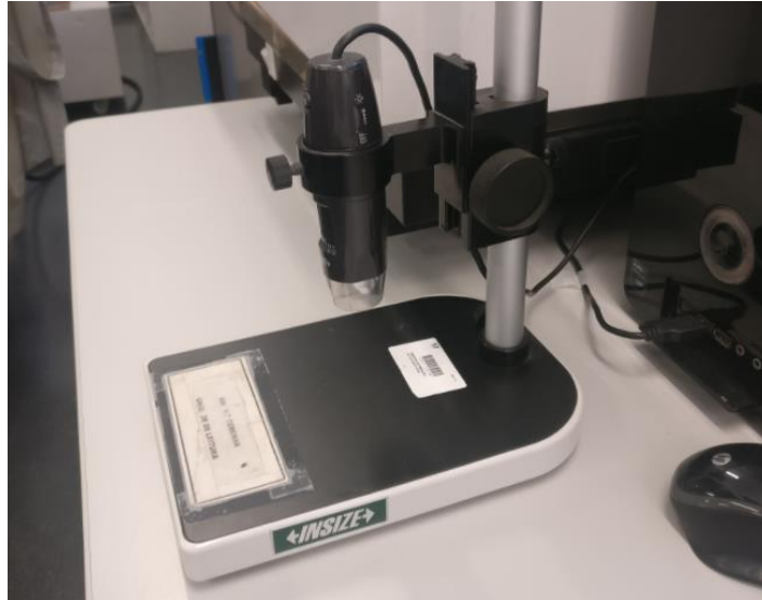
Figure 11 – ISM-PM200S stereomicroscope, utilized in the petrographic analysis of the received natural stone samples.
