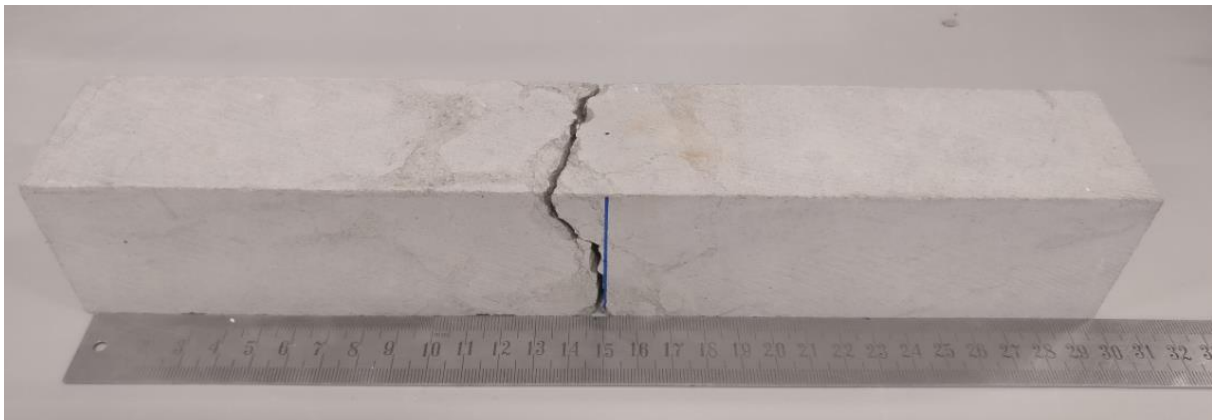
Figure 59 – Limestone AV sample AV19, after being put through the 3-point bending test to determine flexural strength, where it's possible to observe the resulting main fracture follow an already existing set of microfractures.
