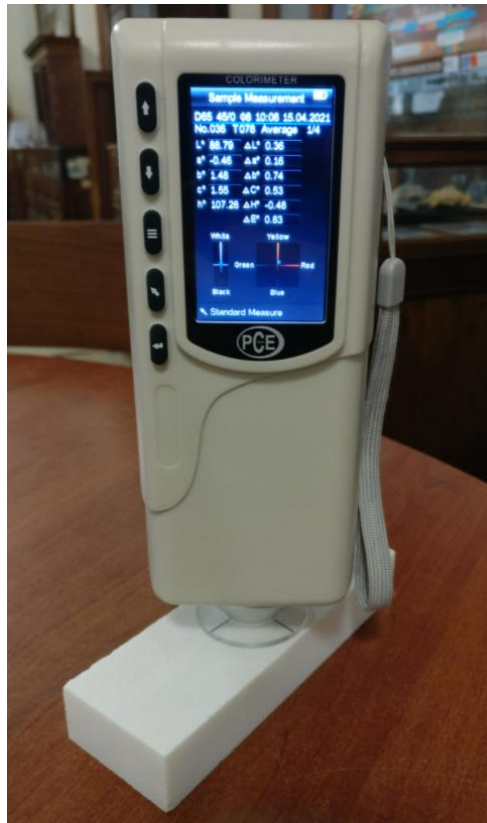
Figure 14 – Measuring of color in the surface of a marble sample, using the handheld colorimeter PCE-CSM 1.
