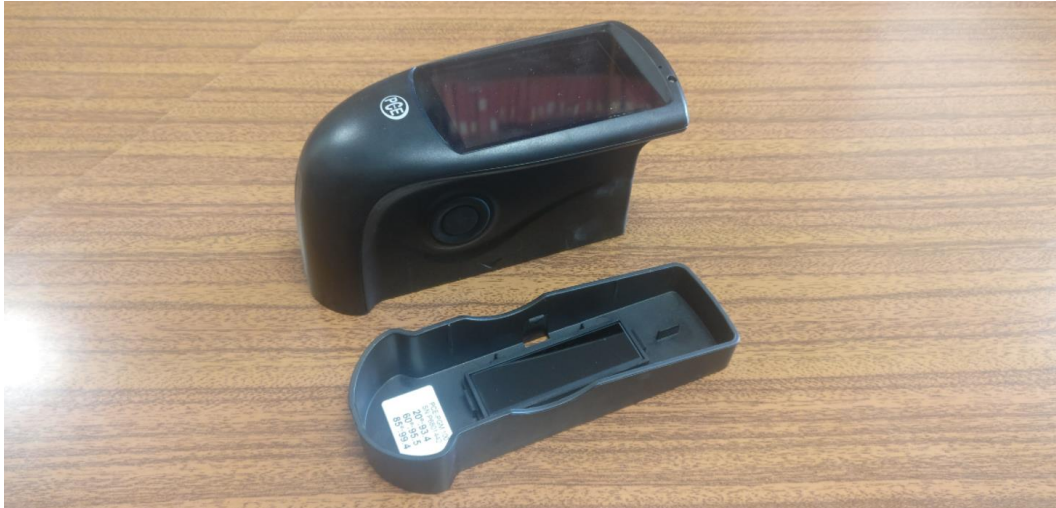
Figure 15 – Gloss Meter PCE-IGM 100 from PCE, utilized in the measuring of gloss on natural stone sample's surfaces.
