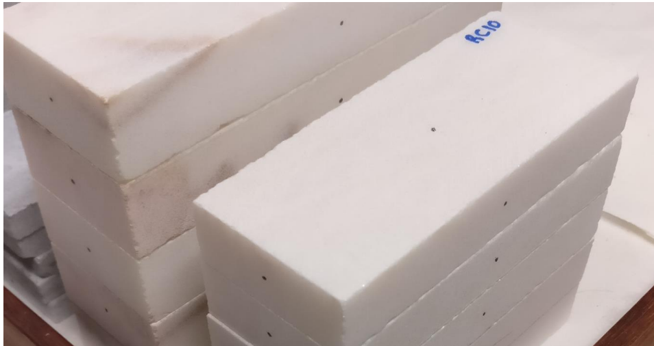
Figure 21 – Example of the marking in the middle of the surfaces of RC Marble samples, on which the exponential transducers were placed in opposing faces, in order to carry out the measuring of P-wave travel time through each sample.
