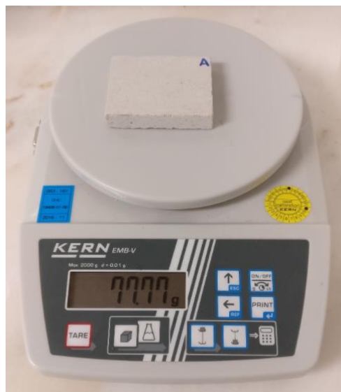
Figure 13 – Digital scale KERN EMB-V, used in the dry weighing and other weighing measurements made throughout the physical testing phase.
