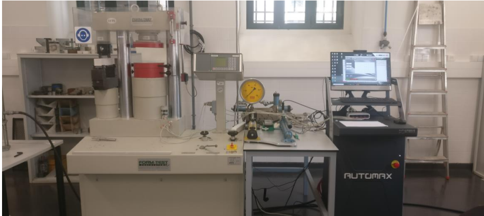
Figure 24 – Hydraulic press FORM-TEST LEHRSYSTEME 506/1000/200 D, a compression and bending testing machine which was used to measure the sample failure load.
